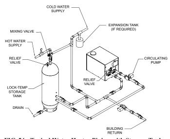
FIG. 54 Typical Water Heater Piping with Storage Tank
